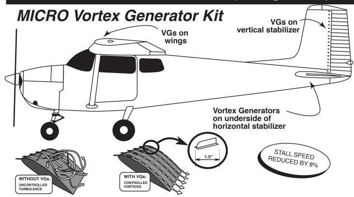
The **MICRO Vortex Generators** for the straight tailed Cessna 172 and 175 are now FAA STC approved and ready for installation on your airplane. This jet age technology provides an 8% reduction in stall speed, improved aileron response, reduced landing and takeoff roll.
